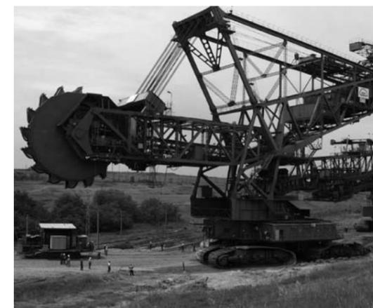
Lignite mining bucket wheel excavator
